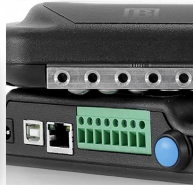
Remote Access Ground Monitor. Connect to a reference Ground and then attach, up to 8 devices where ground is a critical safety concern. Program tolerance via the Free Web Browser software and connect to your network and the OmniGnd will send you and email if any of the grounds fail or exceed tolerance.
